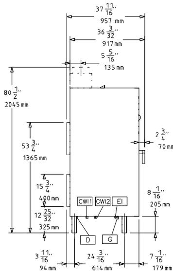
CW11 = Raccordement eau froide      G = Connexion gaz
